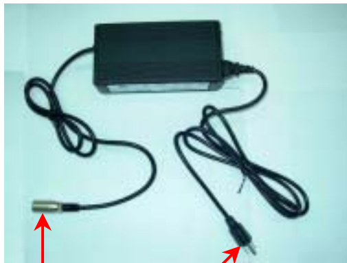
plug-in controller plug-in wall outlet
